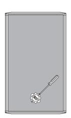
Rotate the RCF Logo 45° to show the two screw heads, then remove the screws.
