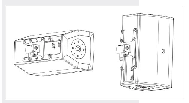
The C3110 models have 8 threaded holes (instead of 6), allowing the direct mounting (without additional bars) of the AC WM-C accessory at the rear panel centre.
