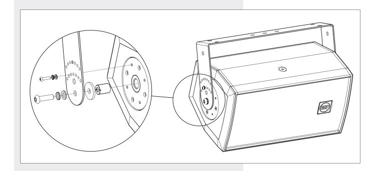
As an alternative, it is possible to install the loudspeaker a bit less prominent, thanks to the U bracket inner holes. Before tightening the two M10 bolts, adjust the loudspeaker vertical tilt and then fix it through two M5x20 bolts into one of the 7 small holes of the U bracket.
