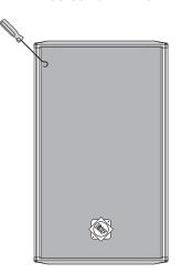
Using a hook, pass through the foam layer and try to locate a hole on a side of the metal grille
