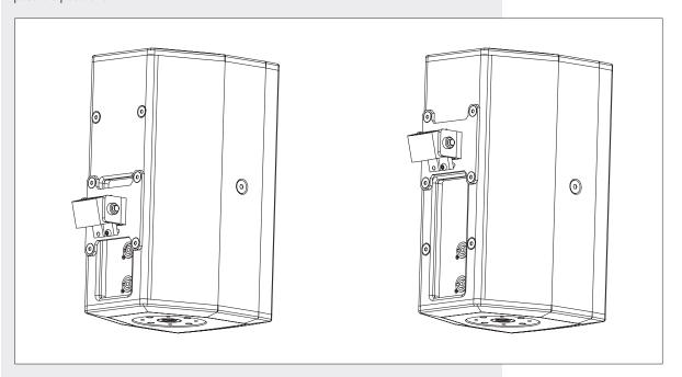
Add the two included bars to mount the swivel bracket at the centre (allowing also a balanced horizontal mounting of the loudspeaker).
