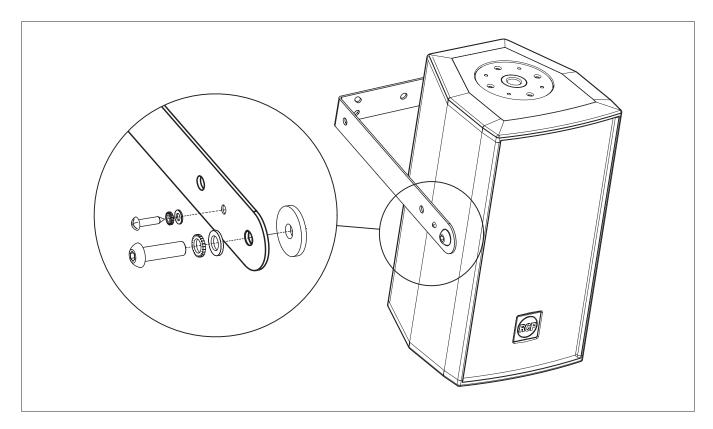
As an alternative, it is possible to install the loudspeaker a bit less prominent, thanks to the U bracket inner holes.
