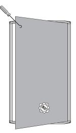
Once the hook is hanged to the metal grille, pull gently. The grille should now lift and can be removed
